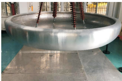
Fig.4 HV electrode (3 m in diameter)
